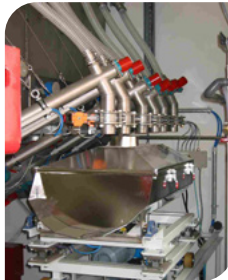
Automatic powder dosing system with movable tipping bucket and scale
