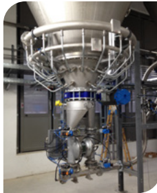
Silo discharge system with DASAG -Powder Pump
